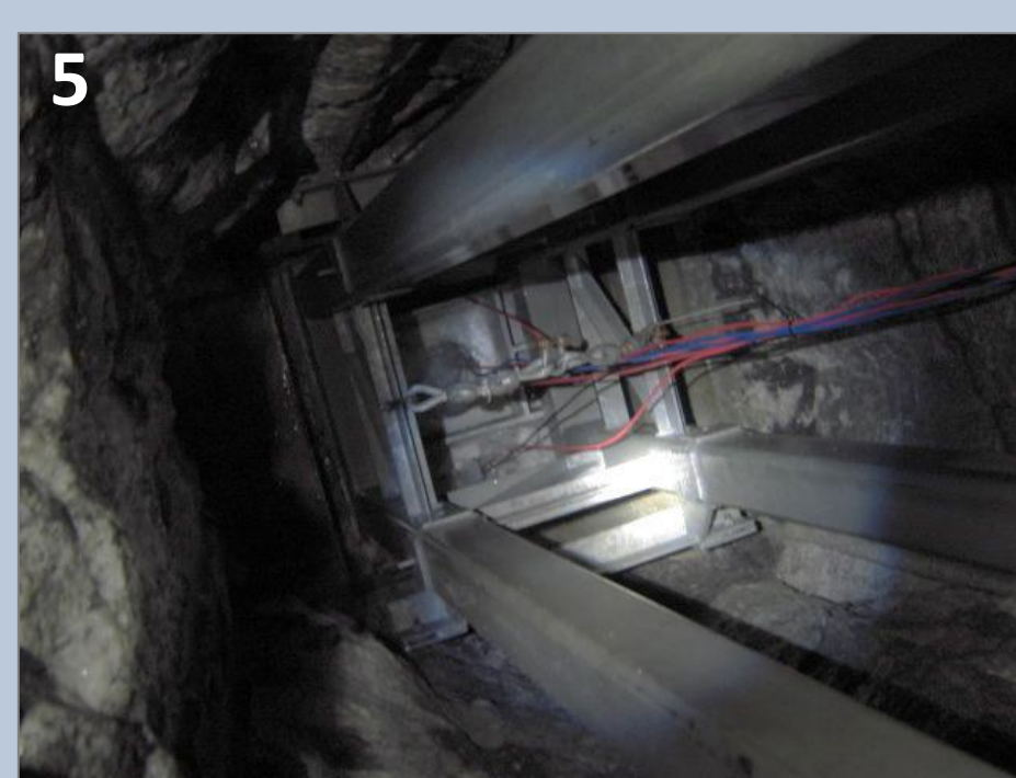
Figure 4. Example of an exposed load cell drilled into the bedrock that sit under the glacier. The cells measure the overall pressure environment experienced at the bed. Note the distinct scours on the metal plate from the debris laden basal ice. Each load cell is approximately the size of a large dinner plate.
